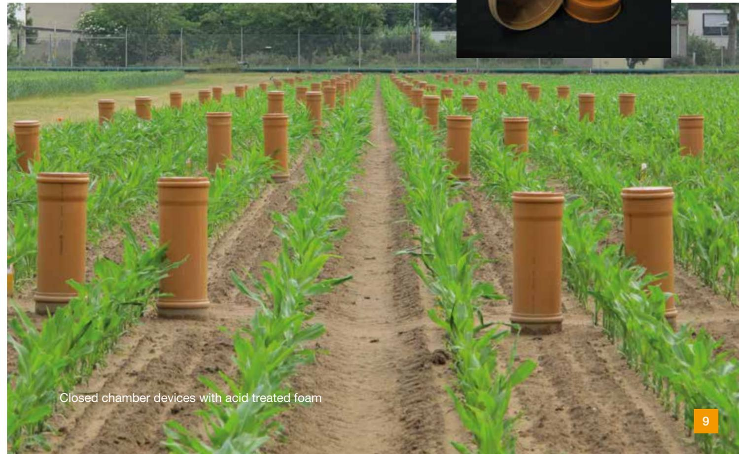
Closed chamber devices with acid treated foam
